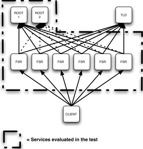
Figure 1: Service topology for the test
